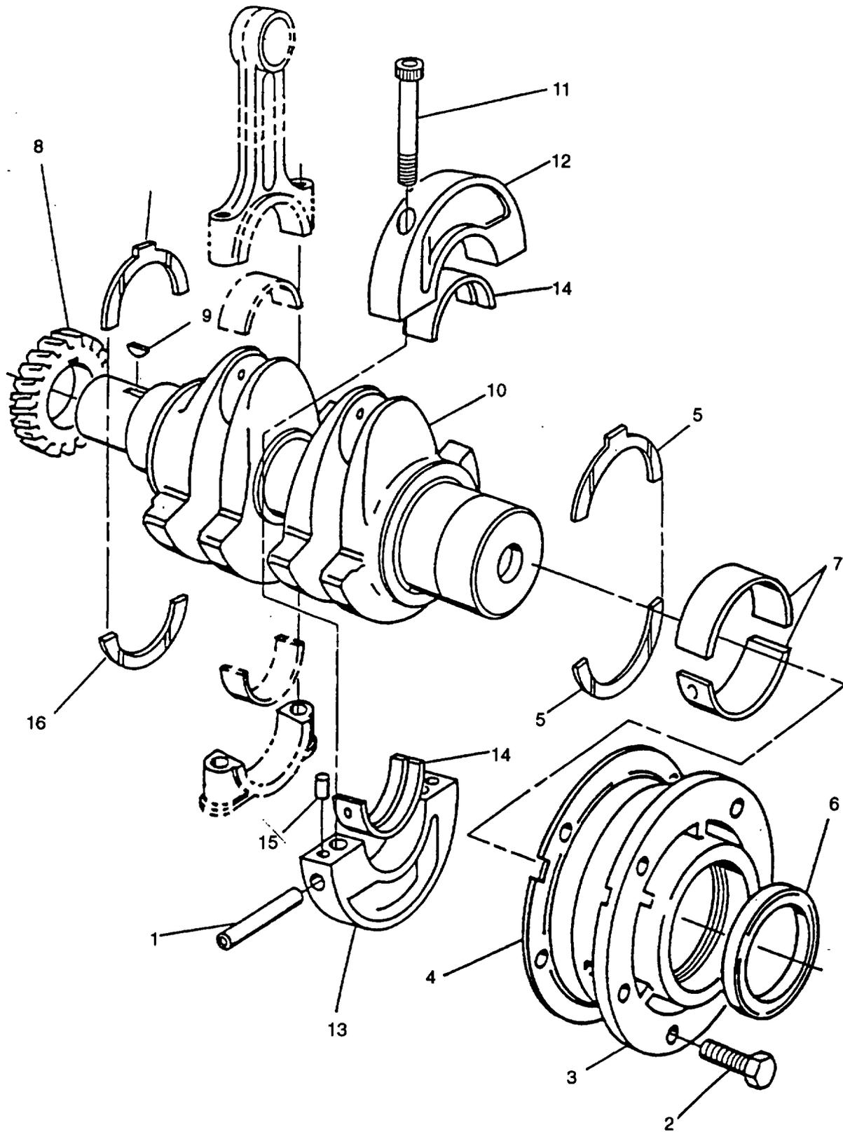
FIGURE 3-40. Crankshaft Assembly
